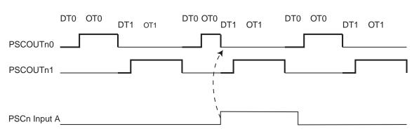
Figure 16-31. PSC behaviour versus PSCn Input A in Mode 8
