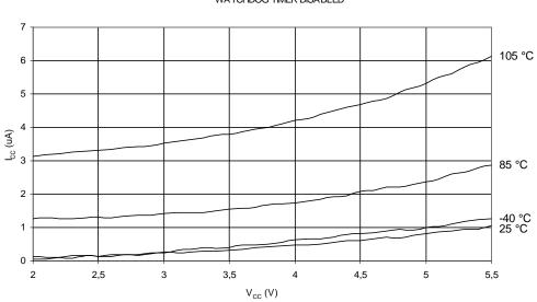
Figure 24-9. Power-Down Supply Current vs. V<sub>CC</sub> (Watchdog Timer Disabled) POWER-DOWN SUPPLY CURRENT vs. V<sub>CC</sub> WATCHDOG TIMER DISABLED
