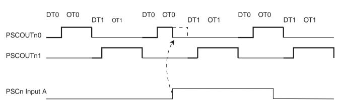
Figure 16-33. PSC behaviour versus PSCn Input A in Mode 9
