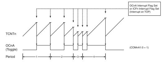
Figure 15-6. CTC Mode, Timing Diagram
