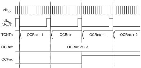
Figure 15-12 shows the count sequence close to TOP in various modes. When using phase and frequency correct PWM mode the OCRnx Register is updated at BOTTOM. The timing diagrams will be the same, but TOP should be replaced by BOTTOM, TOP-1 by BOTTOM+1 and so on. The same renaming applies for modes that set the TOVn Flag at BOTTOM.
