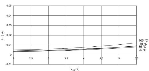
RESET CURRENT vs.  $V_{CC}$  (CLOCK STOPPED) EXCLUDING CURRENT THROUGH THE RESET PULLUP
