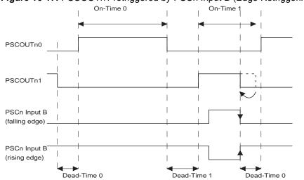
Figure 16-17. PSCOUTn1 retriggered by PSCn Input B (Edge Retriggering)
