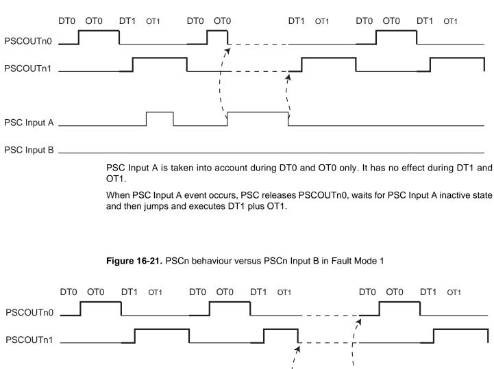
Figure 16-20. PSCn behaviour versus PSCn Input A in Fault Mode 1
