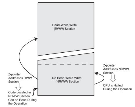
Figure 21-1. Read-While-Write vs. No Read-While-Write
