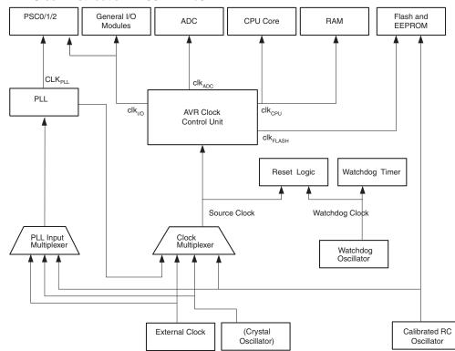
Figure 7-1. Clock Distribution AT90PWM2/3
