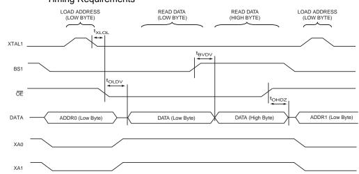
**Figure 22-9.** Parallel Programming Timing, Reading Sequence (within the Same Page) with Timing Requirements<sup>(1)</sup>
