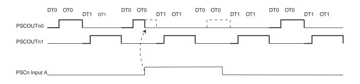
Figure 16-35. PSC behaviour versus PSCn Input A in Mode 14
