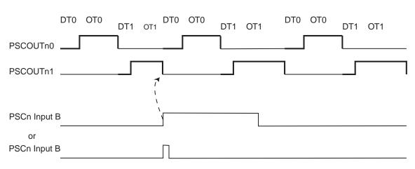
Figure 16-32. PSC behaviour versus PSCn Input B in Mode 8
