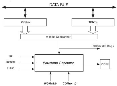
Figure 14-3. Output Compare Unit, Block Diagram
