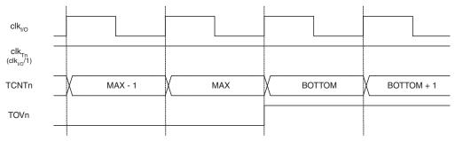
Figure 14-8. Timer/Counter Timing Diagram, no Prescaling
