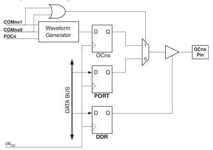
Figure 14-4. Compare Match Output Unit, Schematic
