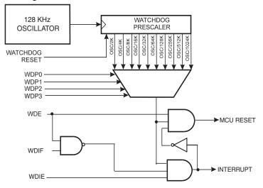
The Watchdog Timer (WDT) is a timer counting cycles of a separate on-chip 128 kHz oscillator. The WDT gives an interrupt or a system reset when the counter reaches a given time-out value. In normal operation mode, it is required that the system uses the WDR - Watchdog Timer Reset - instruction to restart the counter before the time-out value is reached. If the system doesn't restart the counter, an interrupt or system reset will be issued.
