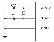
The Oscillator can operate in three different modes, each optimized for a specific frequency range. The operating mode is selected by the fuses CKSEL3..1 as shown in Table 7-3.
