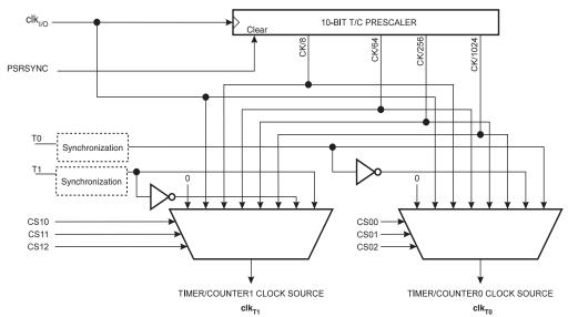
Figure 13-2. Prescaler for Timer/Counter0 and Timer/Counter1<sup>(1)</sup>
