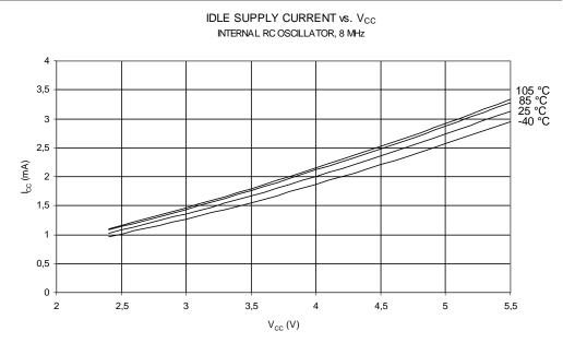
Figure 24-7. IIdle Supply Current vs. V<sub>CC</sub> (Internal RC Oscillator, 8 MHz)
