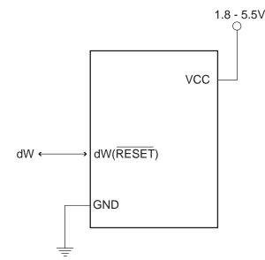
Figure 20-1. The debugWIRE Setup
