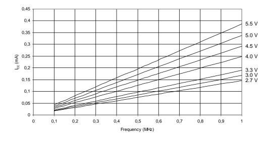
Figure 24-5. Idle Supply Current vs. Frequency (0.1 - 1.0 MHz) IDLE SUPPLY CURRENT vs. LOW FREQUENCY
