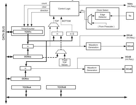
Figure 14-1. 8-bit Timer/Counter Block Diagram
