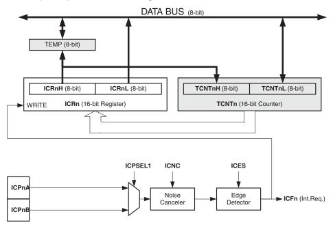
Figure 15-3. Input Capture Unit Block Diagram
