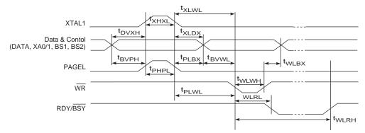
Figure 22-8. Parallel Programming Timing, Loading Sequence with Timing Requirements<sup>(1)</sup>
