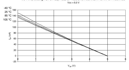
**Figure 24-11.** I/O Pin Pull-Up Resistor Current vs. Input Voltage (V<sub>CC</sub> = 5V) VO PIN (including PE1 & PE2) PULL-UP RESISTOR CURRENT vs. INPUT VOLTAGE
