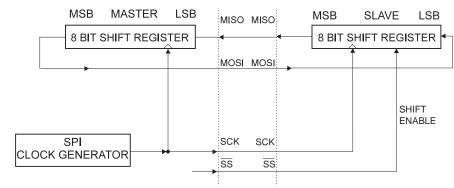
Figure 17-2. SPI Master-slave Interconnection
