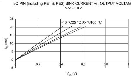
Figure 24-17. I/O Pin Sink Current vs. Output Voltage ( $V_{CC} = 5V$ ) I/O PIN (including PE1 & PE2) SINK CURRENT vs. OUTPUT VOLTAGE
