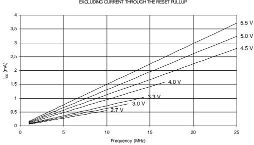
RESET SUPPLY CURRENT vs.  $V_{CC}$  EXCLUDING CURRENT THROUGH THE RESET PULLUP
