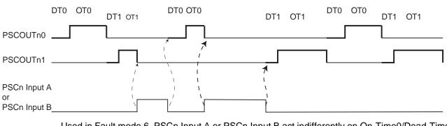
Figure 16-29. PSC behaviour versus PSCn Input A in Fault Mode 6
