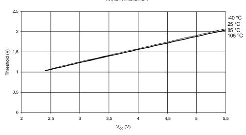
Figure 24-19. I/O Pin Input Threshold Voltage vs. V<sub>CC</sub> (VIH, I/O Pin Read As '1') I/O PIN (including PE1 & PE2) INPUT THRESHOLD VOLTAGE vs. V<sub>CC</sub> VIH, IO PIN READ AS '1'
