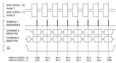
**Figure 17-4.** SPI Transfer Format with CPHA = 1
