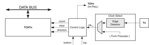
Figure 14-2. Counter Unit Block Diagram
