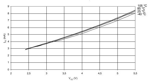
Figure 24-3. Active Supply Current vs. V<sub>CC</sub> (Internal RC Oscillator, 8 MHz) ACTIVE SUPPLY CURRENT vs. V<sub>CC</sub> INTERNAL RC OSCILLATOR, 8 MHz
