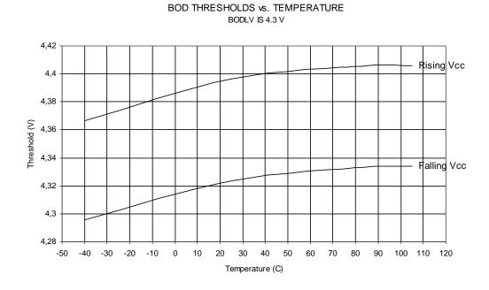
Figure 24-29. BOD Thresholds vs. Temperature (BODLEVEL Is 4.3V)
