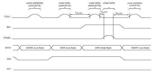
Note: 1. The timing requirements shown in Figure 22-7 (i.e., t<sub>DVXH</sub>, t<sub>XHXL</sub>, and t<sub>XLDX</sub>) also apply to loading operation.
