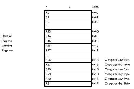
Figure 5-2. AVR CPU General Purpose Working Registers
