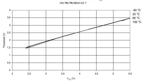
Figure 24-27. PE0 Input Threshold Voltage vs.  $V_{CC}$  (PE0 Pin Read As '1') PE0 INPUT THRESHOLD VOLTAGE vs.  $V_{cc}$
