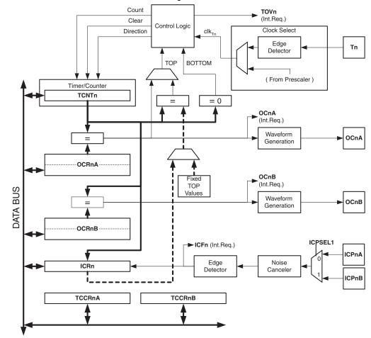
**Figure 15-1.** 16-bit Timer/Counter Block Diagram<sup>(1)</sup>
