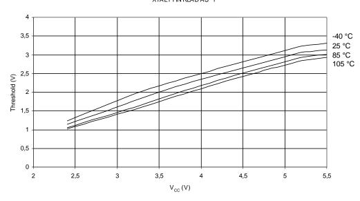
Figure 24-25. XTAL1 Input Threshold Voltage vs. V<sub>CC</sub> (XTAL1 Pin Read As '1') XTAL1 INPUT THRESHOLD VOLTAGE vs. V<sub>CC</sub> XTAL1 PIN READ AS "1"
