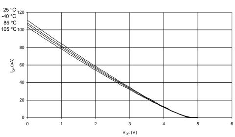
Figure 24-13. Reset Pull-Up Resistor Current vs. Reset Pin Voltage ( $V_{CC} = 5V$ ) PE0 and RESET PULL-UP RESISTOR CURRENT vs. INPUT VOLTAGE Vcc = 5.0 V
