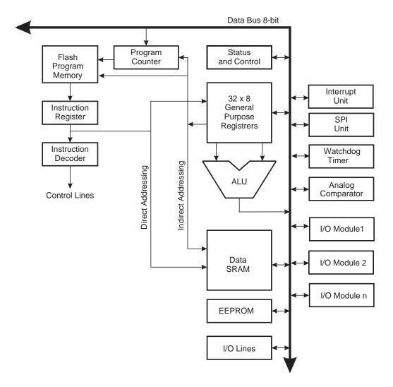
Figure 5-1. Block Diagram of the AVR Architecture
