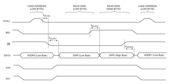
Note: 1. ggThe timing requirements shown in Figure 23-5 (i.e., t<sub>DVXH</sub>, t<sub>XHXL</sub>, and t<sub>XLDX</sub>) also apply to reading operation.
