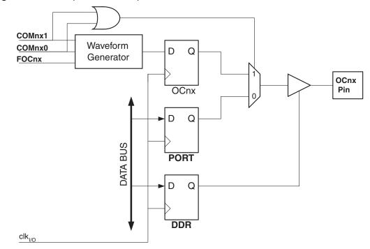
Figure 15-5. Compare Match Output Unit, Schematic
