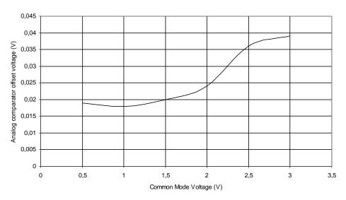
Note: corrected on AT90PWM2B/3B to allow almost full scale use.
