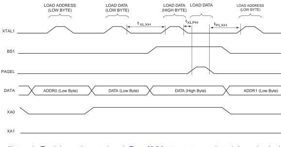
Note: 1. The timing requirements shown in Figure 23-5 (i.e., t<sub>DVXH</sub>, t<sub>XHXL</sub>, and t<sub>XLDX</sub>) also apply to loading operation.
