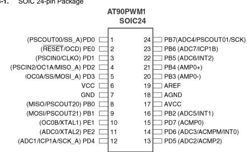
Figure 3-1. SOIC 24-pin Package
