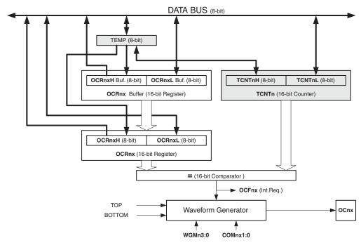
Figure 15-4. Output Compare Unit, Block Diagram
