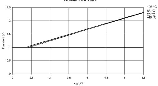
Figure 24-23. Reset Input Threshold Voltage vs. V<sub>CC</sub> (VIL, Reset Pin Read As '0') RESET INPUT THRESHOLD VOLTAGE vs. V<sub>CC</sub> VIL, RESET PIN READ AS '0'
