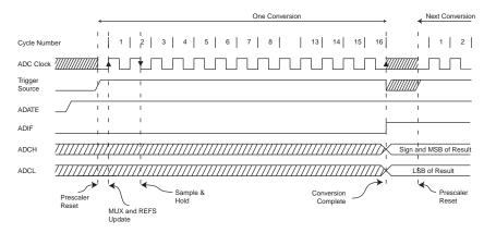
Figure 19-7. ADC Timing Diagram, Free Running Conversion
