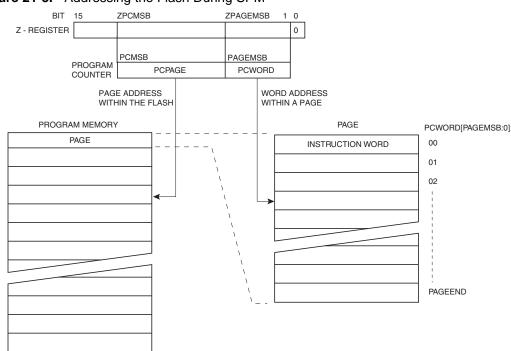
**Figure 21-3.** Addressing the Flash During SPM<sup>(1)</sup>
