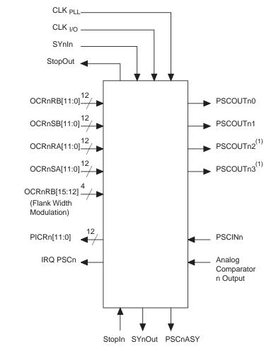
Figure 16-3. PSC External Block View
