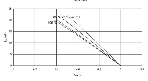
Figure 24-15. I/O Pin Source Current vs. Output Voltage ( $V_{CC}$  = 5V) I/O PIN (including PE1 & PE2) SOURCE CURRENT vs. OUTPUT VOLTAGE Vcc = 5.0 V
