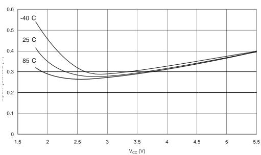
Figure 24-21. I/O Pin Input HysteresisVoltage vs. V $_{\rm CC}$  I/O PIN INPUT HYSTERESIS vs. V $_{\rm CC}$
