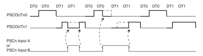
Figure 16-26. PSC behaviour versus PSCn Input A or Input B in Mode 4
