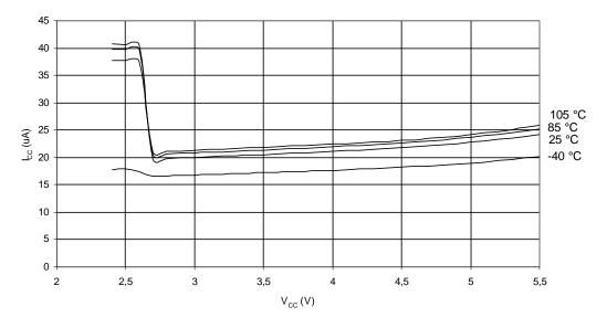
Figure 24-40. ADC Current vs. V<sub>CC</sub> (ADC at 50 kHz)
