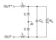
The cut off frequency fc of the output LC filter is calculated by the following formula.
