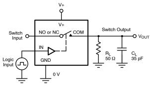
C<sub>L</sub> (includes fixture and stray capacitance)
