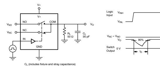
FIGURE 3. Break-Before-Make Interval
